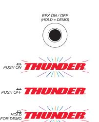
NOTE: Demo mode is usable with the amplifier on or off, and will draw current until turned off manually.
