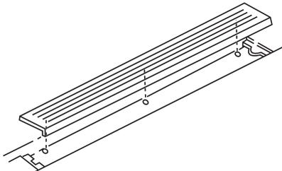
4. Using furnished wiring harness route 10ga red power wire starting at pre-amp location. Route wire on driver's side, over to threshold and under
