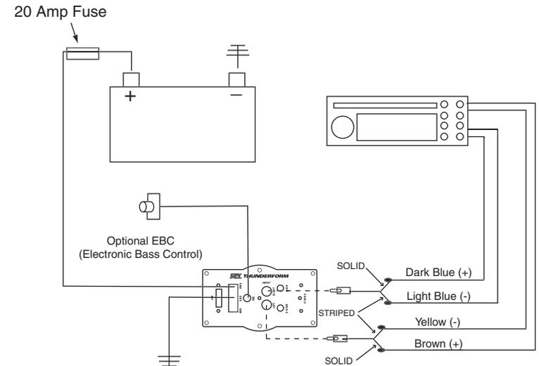
19. Plug power wire harness into amplifier pre-amp.
