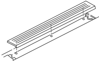
25. Using screws provided, install the enclosure into vehicle as shown below.
