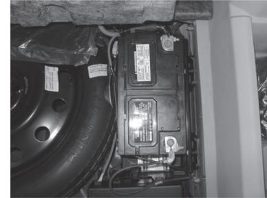
7. Ground amplifier to chassis of vehicle; connect the terminal provided to the 10ga black wire from furnished wiring harness. A good ground is as important as the power connection. The ground should be as short as possible and the contact point should be free of paint and debris.
