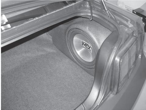
2. Make note of the terminal/pre-amp location and then move enclosure aside to route wires to that location.
