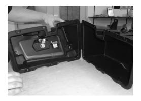
Step 11 - Cut the "binding" plastic hinge with a razor knife to separate the front and back of the glove box. The back side of the glove box will no longer be used. The front side of the glove box will be attached to the enclosure.
