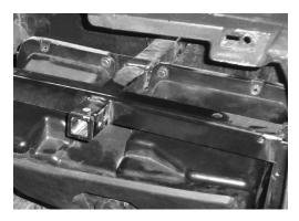
Step 10 - Remove the five (5) T25 screws holding the glove box together. The glove box will then open like a book.
