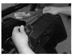
Step 8 - Carefully lift the dash out of the vehicle. If the locking clips have fallen off, place them back onto the locking tabs on the dash. These are needed to re-assemble the dashboard.
