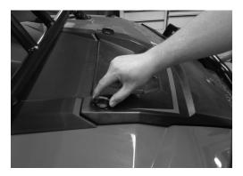
Step 2 - Lift up the hood and slide towards the front of the vehicle.
