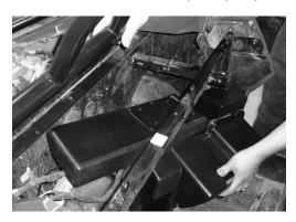
Step 14 - Hold the enclosure up and align the glove box screw holes with the vehicle frame mount. Replace the two (2) 10mm hex bolts and tighten the enclosure in place. It may help to place a supporting object under the enclosure so both hands are free to line up the screw holes with the vehicle frame mount.
