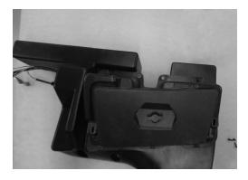
Step 13 - The enclosure can now be placed into the vehicle. Place the rectangular protrusion at an angle into the dash area first. The enclosure can then easily slide up into place.
