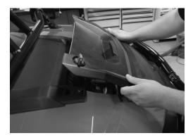
Step 3 - Remove the two (2) T40 screws holding down the top dash cover.
