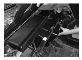
Step 15 - There are three mounting holes on the bottom of the enclosure to screw the base of the enclosure into place. The furthest hole to the right uses the included 1" screw. The other two mounting holes use the 1.5" screws. Tighten the screws down, but take care to not strip them. These screws lock into the plastic foot board.
