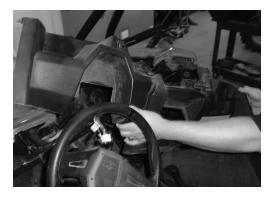
Step 9 - Remove the two (2) 10mm hex bolts that are holding the glove box to the vehicle frame. When the screws are removed the glove box can be lowered down and out of the enclosure.
