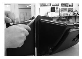
Step 12 - Using the five (5) T25 screws that were removed from the front / back assembly of the glove box, attach the front of the glove box to the RZRXP-10 enclosure. Take care to not strip out the plastic, but tighten it enough so the enclosure and glove box are solidly connected.
