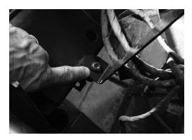
Step 6 - Remove the two (2) T40 screws holding the dashboard in place.
