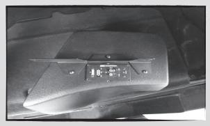
Attach the mounting bracket to the enclosure as shown using the supplied hardware.
