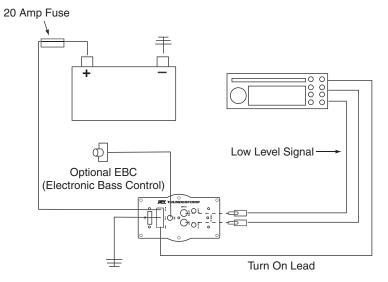
**Optional-** The EBC, or Electronic Bass Control, allows a remote bass control to be adjusted from the driver's seat.
