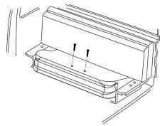
22. First remove passenger side threshold. Remove the cover on rear seat mounting bracket on passenger side. Pull out the two push in fasteners. Now you can lift up carpet and remove jack bracket. There are (2) 15mm and (1) 10mm bolt. (Save bracket and hardware, if you sell or trade the truck you may want to replace it.)
