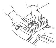
**13**. Ground amplifier to chassis of vehicle; connect the terminal provided to the 10ga black wire from furnished wiring harness. A good ground is as important as the power connection. The ground should be as short as possible and the contact point should be free of paint and debris.
