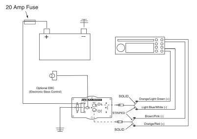
**15.** Plug power wire harness into amplifier pre-amp.
