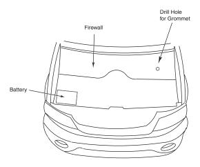
Note: To avoid any damage to parts inside engine compartment, drill from inside of vehicle using a short bit.
