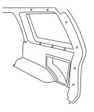
**9**. If vehicle was equipped with factory amplified subwoofer system remove three 11/32" bolts holding it into place. Unplug amplifier and remove enclosure.
