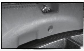
Remove the three clips that hold the rear sill panel in place. Carefully pull up on the panel to release the remaining clips. Remove the sill panel from the vehicle.
