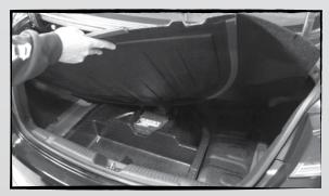
Locate and remove the Phillips head screw holding the trunk floor. Remove the trunk floor from the vehicle.
