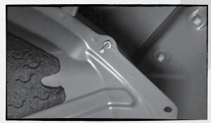
Slide the  $5\!/_{16}$  - 18x1 bolt through the enlarged hole. Place the lock washer and nut on the bolt and tighten.
