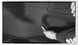
Cut an "X" into the trunk liner, allowing the bolt to pass through. Reinstall the three clips and Phillips head screw to hold the trunk liner in place. Reinstall the sill panel and trunk floor.
