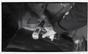
Locate the upper hole in the metal brace. Using a  $5\!\!/_6$  drill bit, enlarge the hole.
