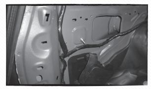
With the interior panel removed, note the location of the hole you just drilled. Place the bolt from the mounting hardware into the hole from the back side. Install a flat washer, lock washer, a nut, and tighten. This will form a stud for the enclosure to mount to.
