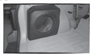
Remove the woofer from the enclosure. Set enclosure in place as shown. Using the hole in the back of the enclosure as a guide, place a mark on the interior panel behind the enclosure. This will be used to mount the enclosure. Drill a hole in the interior panel where marked as shown.
