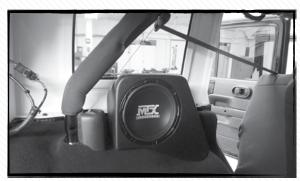
Make all final wire connections, and mount the enclosure into place using the bolts removed from the rooftop in Step 1.
