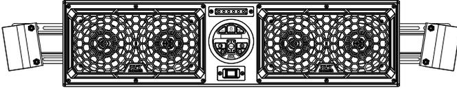
Physical Dimensions - 8.5" (216mm)H x 4.125" (105mm)D x 29.92" (760mm)W
