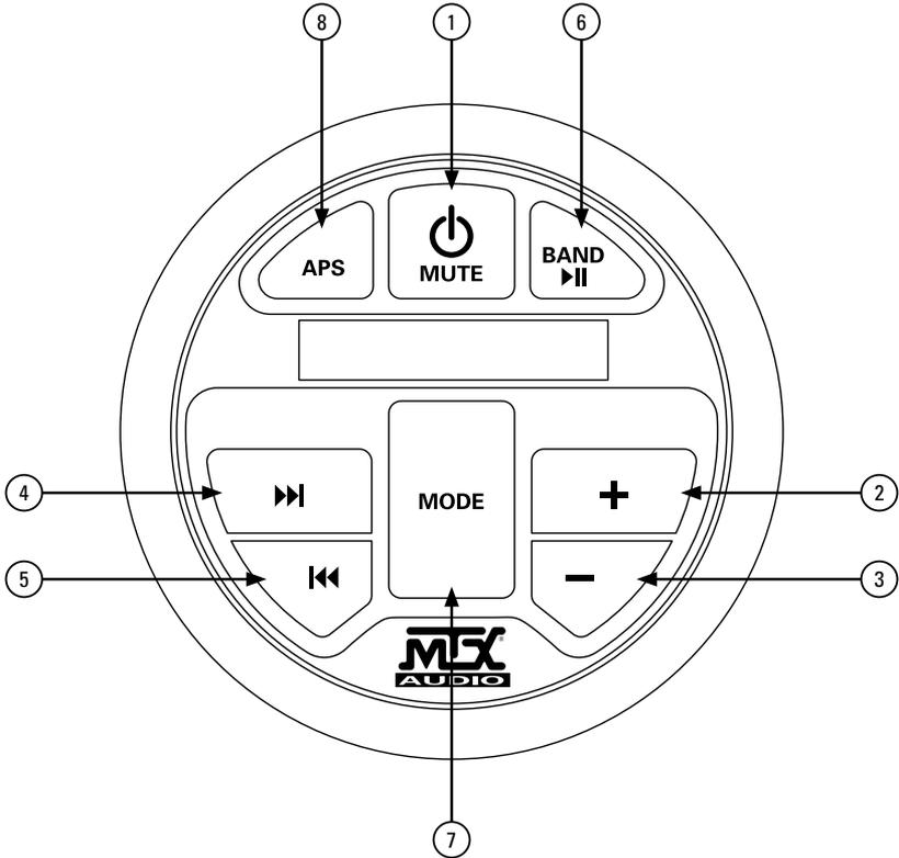
1. Power / Mute Button - Press the button to turn power On. When the power is On, press the button to mute the audio output. Press and hold the button to turn power Off.
