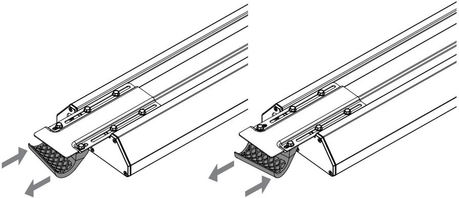
Each C-bracket has two (2) total bolts. These bolts can be loosened to adjust the clamp angle allowing it to mount to a variety of roll cages including those that are angled.
