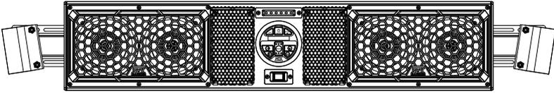
Physical Dimensions - 8.5" (216mm)H x 4.125" (105mm)D x 40.5" (1029mm)W
