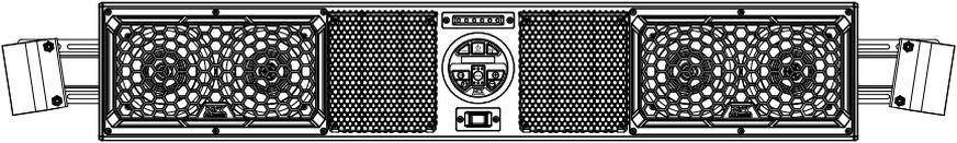
Physical Dimensions - 8.5" (216mm)H x 4.125" (105mm)D x 46.813" (1189mm)W
