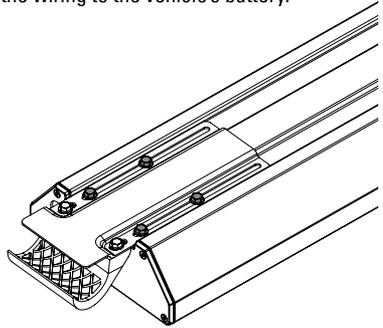
When the bolts are loosened, the bracket can slide to accommodate a variety of roll cages whose inside roll bar dimension is between 32.25" and 38.75" for the MUDSYS31, 43.0" and 49.0" for the MUDSYS41, and 49.25" and 56.0" for the MUDSYS46. Once the proper width has been established, these bolts should be retightened to a torque specification of 40-45 inch/lbs.
