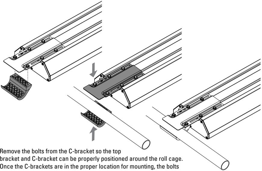
Remove the bolts from the C-bracket so the top bracket and C-bracket can be properly positioned around the roll cage. Once the C-brackets are in the proper location for mounting, the bolts should be retightened to a torque specification of 65-70 inch/lbs.
