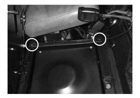
Step 7 - Remove the two T40 screws as shown above. These screws hold down the vehicle plastic brace under the seat.
