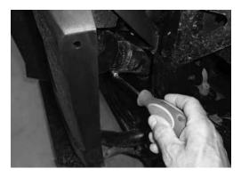
Step 5 - Carefully pull away the side panel from vehicle. The gas cap / fuel filler pipe is attached to the plastic side panel and will slide out of the rubber fuel pipe.
