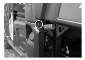
The **dual cab RANGER** uses two screws on the floor area, one screw on the fascia below the seat, and one screw on the back of the side panel.
