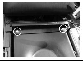
Step 9 - Line up the brass insert on the front of the enclosure with the hole in the vehicle frame. Using the included M6 bolt and washer, attach the enclosure to the vehicle.
