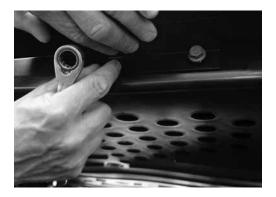
Step 12 - Attach the enclosure to the 90° angle bracket using the included ST6.3 self-tapping screws. A ¼" drill bit should be used to pre drill holes in the enclosure. Be careful not to strip them when tightening into the enclosure material. Do not use an impact driver for these screws.
