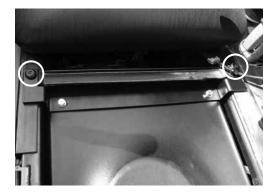
Attach the bracket to the two brass inserts in the top of the enclosure using the included M6 bolts and washers, hand tighten.
