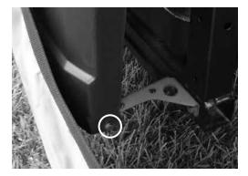
Step 4 - Loosen the pipe clamp on the fuel filler pipe with a flat blade screw driver. The fuel filler pipe should be able to be pulled from the rubber fuel pipe. Take care when doing so. **WARNING**: Do not smoke during this step.
