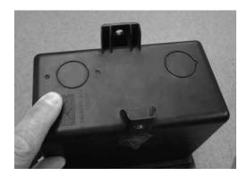
Step 13 - Attach the dash kit to the center pocket by first inserting the wiring into the pocket. Connect the wiring to the source unit and feed the wiring out of the rear of the pocket hole that was cut. Place the dash kit onto the front of the pocket.
