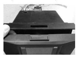
Step 15 - Once the dash kit is locked in, use the two included shoulder bolts to attach the bottom of the dash kit to the pocket.
