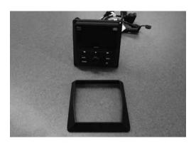
Step 11 - Attach the source unit to the rear of the dash kit using the included nuts.
