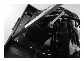
Step 12 - One of the circular knockout panels on the rear of the pocket will need to be removed to provide an access hole to route wiring from the source unit to the vehicle.
