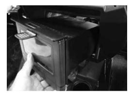
Step 7 - Turn the center pocket upside down to access the protective cover pins. Pry the two pins loose using a pry tool to remove the cover.
