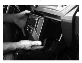
Step 17 - Reattach the rear support bracket to the pocket. Once rear brace is secure, the dash kit is installed and the vehicle can be put back together.
