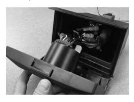
Step 14 - Insert the tab on top of the dash kit into the slot on the pocket.
