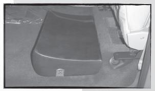
Flip up the driver side rear seat and place the enclosure on the floor as shown above. The enclosure should be even with the edge of the seat when the seat is in the lowered position.
