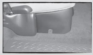
Attach the mounting bracket to the enclosure as shown using (2) 2" screws to attach the bracket to the floor, and (1) M6 bolt to attach the bracket to the enclosure.
