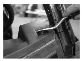
Step 3 - Lift and pull back the top dash cover to release the clips holding it in place.
