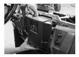
Step 8 - Mount the dash kit using the two (2) T-20 screws removed earlier.
