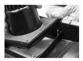
Step 6 - With the radio seated in place, install four (4) included retaining nuts using a 5.5mm socket or nut driver
