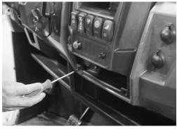
Step 5 - Prepare the new dash kit by aligning the radio with the four (4) pre-installed threaded posts.
