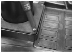
Note: This dash kit also offers space to mount additional rocker panel switches for accessories. On the rear of the dash kit, grooves are provided to give you proper location and size for mounting.
