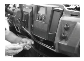
Step 9 - Reinstall the top dash panel and reattach using the hardware removed earlier.
