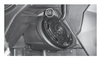
Step 7 - Feed wire into dash towards amplifier mounting location. **Note:** In the event these are not used with an MTX THUNDER SYSTEM, it will be necessary to cut off the connectors and hardwire directly to your equipment.
