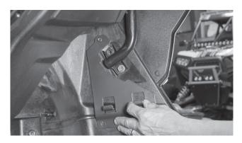
Step 4 - Reinstall the body bolt and two (2) T40 screws.
