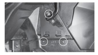
Step 5 - Align the bottom of the RZR-14-FS speaker pod with the hooks on the custom quick mount speaker bracket. Tilt the top of the speaker pod toward the outer body until flush against the mounting bracket. Push down until the pod locks in place.
