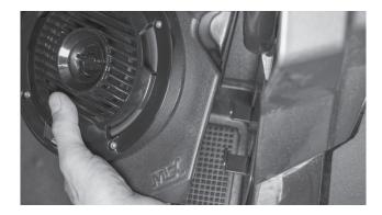
Step 6 - Align the top of the speaker pod with the speaker bracket and insert the supplied 10mm bolt.
