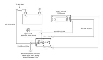
Step 16 - Plug power wire harness into amplifier pre-amp.
