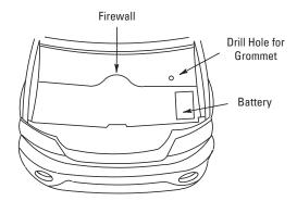
Step 9 - Route 10ga red power wire through grommet into the engine compartment.
