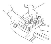
Step 13 - Ground amplifier to chassis of vehicle; connect the terminal provided to the 10ga black wire from furnished wiring harness. A good ground is as important as the power connection. The ground should be as short as possible and the contact point should be free of paint and debris.
