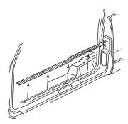
Step 5 - Remove driver side kick panel, grasp center upper edge and pull outward allowing retaining tab to unsnap.
