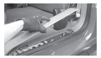
Step 5 - Using the furnished wiring harness route 10ga red power wire starting at pre-amp location. Route wire on driver side, over to threshold and under carpet to the front of vehicle.
