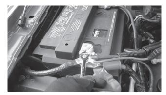
Step 12 - Ground amplifier to chassis of vehicle; connect the terminal provided to the 10ga black wire from furnished wiring harness. A good ground is as important as the power connection. The ground should be as short as possible and the contact point should be free of paint and debris.
