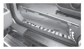
Step 4 - Remove rear driver door threshold trim. Pull up on trim; it will remove easily.
