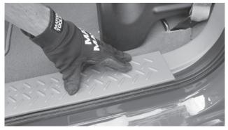
Step 20 - Screw enclosure to bracket (with rear driver door open you can screw enclosure to bracket easily). Make sure enclosure is tight against the bottom of the seat.
