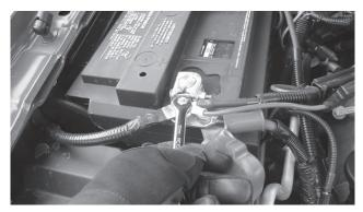
Step 13 - Ground amplifier to chassis of vehicle; connect the terminal provided to the 10ga black wire from furnished wiring harness. A good ground is as important as the power connection. The ground should be as short as possible and the contact point should be free of paint and debris.
