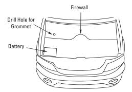
Step 8 - Drill a hole through the fire wall. Locate a spot low on the fire wall on the passenger side. You should always look to find a clear path. Drill a hole from inside of the vehicle into engine compartment and insert grommet. You may also find a pre-existing, unused rubber grommet in this location that you can pass the wire through. **Note:** To avoid any damage to parts inside engine compartment, drill from inside of vehicle using a short bit.
