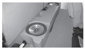
Step 22 - Using the supplied hardware, secure the enclosure to floor of vehicle as shown below.
