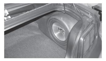
Step 2 - Make note of the terminal / pre-amp location and then move enclosure aside to route wires to that location.
