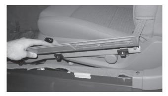
Step 6 - Using furnished wiring harness route 10ga red power wire starting at pre-amp location. Route wire under rear seat on driver side, over to threshold and under carpet to the front of vehicle.
