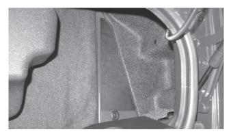
Step 22 - Place enclosure into corner of trunk with its front edge over the folded section of the floor mat. Make sure the enclosure is pressed firmly against the side walls of the truck liner and tail light.
