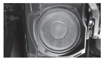
Step 3 - Remove two (2) T-27 screws found at the back of the speaker pod on the firewall.
