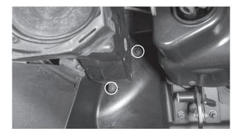
Step 4 - Remove one (1) T-40 Bolt from the inside fender well.
