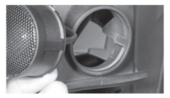
Step 21 - Press the tweeter into the opening from behind until the grille is seated flush with the front of the enclosure.
