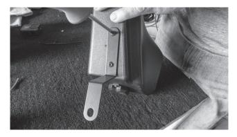
Step 14 - Placing the Speaker enclosure against the dash housing from the rear and holding it in place, loosely install four (4) 30mm T-20 TORX screws from the front into the enclosure housing in the predrilled holes.
