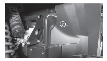
Step 5 - Disconnect the speaker pod plug and remove the pod from the vehicle.
