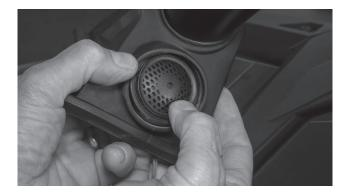
Step 11 - If OE tweeter is installed, disconnect the harness connector.
