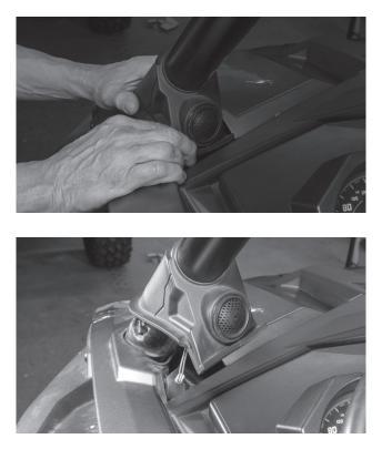
Step 10 - Press the dummy plug or OE tweeter if installed from the front and remove from the enclosure from the rear.
