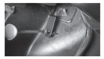
Step 16 - Tighten the four (4) screws on the front of the enclosure.
