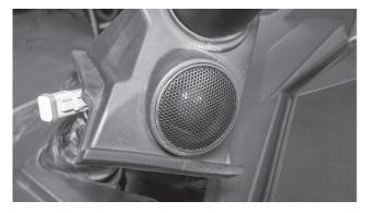
Step 22 - Connect the harness connector from the lower speaker enclosure to the tweeter harness.
