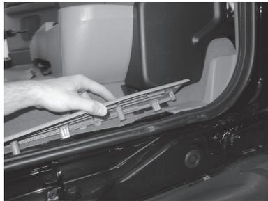
6. Using furnished wiring harness route 10ga red power wire starting at pre-amp location. Route wire on drivers side, over to threshold and under carpet to the front of vehicle.
