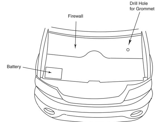
8. Drill a hole through the fire wall. Locate a spot low on the fire wall on the passenger side. You should always look to find a clear path. Drill a hole from inside of the vehicle into engine compartment and insert grommet. You may also find a pre-existing, unused rubber grommet in this location that you can pass the wire through.
