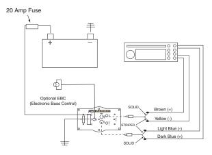
**16.** Plug power wire harness into amplifier pre-amp.
