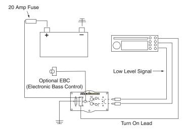
**9.** Route 10ga red power wire through a grommet into the engine compartment.
