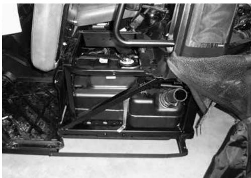
Step 6 - Slide the long part of the enclosure into the vehicle frame above the gas tank. The subwoofer will face the top of the gas tank. Two brass inserts will be visible when looking down from the top and the MTX logo will be pointing towards the outside of the vehicle.
