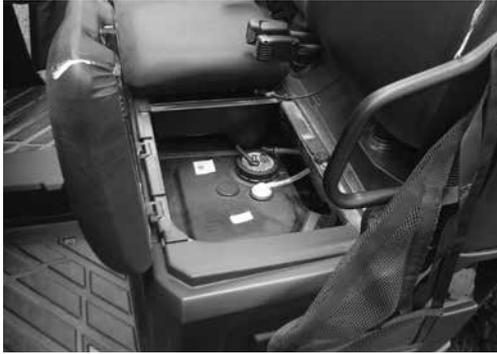
Step 2 - Remove the T40 screws from the driver's side. The **single cab RANGER** uses four screws on the floor area, one screw on the front fender area (the lowest screw), and one screw on the back of the side panel.
