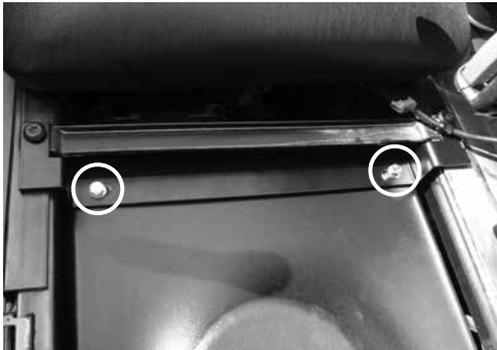
Step 9 - Line up the brass insert on the front of the enclosure with the hole in the vehicle frame. Using the included M6 bolt and washer, attach the enclosure to the vehicle.
