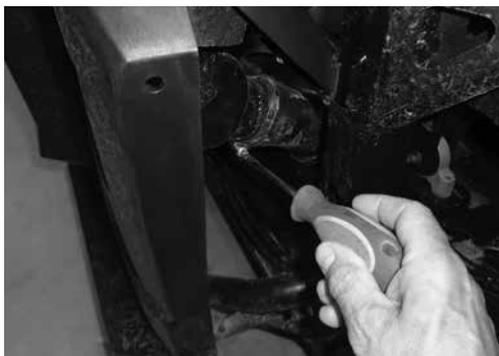
Step 5 - Carefully pull away the side panel from vehicle. The gas cap / fuel filler pipe is attached to the plastic side panel and will slide out of the rubber fuel pipe.
