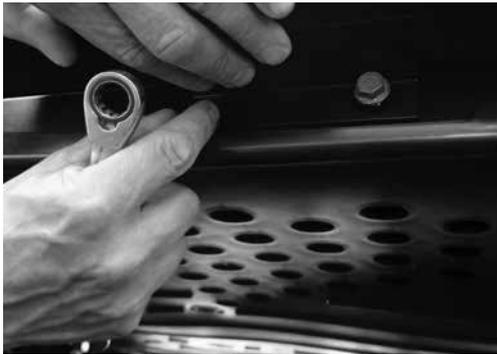
Step 12 - Attach the enclosure to the 90° angle bracket using the included ST6.3 self-tapping screws. A 1/8" drill bit should be used to pre drill holes in the enclosure. Be careful not to strip them when tightening into the enclosure material. Do not use an impact driver for these screws.
