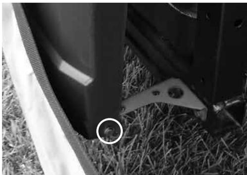
Step 4 - Loosen the pipe clamp on the fuel filler pipe with a flat blade screw driver. The fuel filler pipe should be able to be pulled from the rubber fuel pipe. Take care when doing so.
