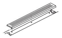
**3.** Remove driver side threshold trim; pull up on trim, it will remove easily.
