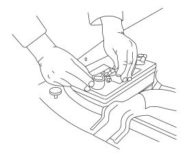
**12**. Ground amplifier to chassis of vehicle; connect the terminal provided to the 10ga black wire from furnished wiring harness. A good ground is as important as the power connection. The ground should be as short as possible and the contact point should be free of paint and debris.
