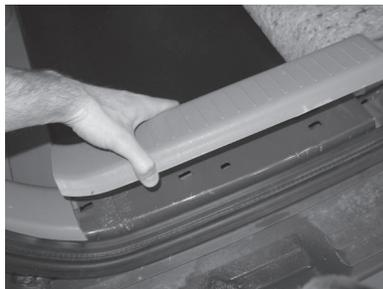
5. From the back side of the quarter panel, use a soldering iron or hot knife to melt the clips holding in the storage pocket. Set the cover in a safe spot because it can be glued back into place if the enclosure is ever removed.
