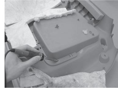
**6.** Reinstall the rear quarter panel. Reverse the steps of removal. Leave the cargo net hanger out. It will be reinstalled later in step 27.
