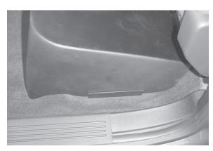
Place one bracket under and against enclosure as shown above. Move enclosure out of the way, making sure bracket doesn't move. Using (2) of the 2" screws from the supplied hardware, secure bracket to floor. (NOTE: When securing bracket to floor, make sure to check floor, and underside of vehicle for wire or objects). Move enclosure back into place against the now secured bracket and using (2) of the 1" screws from the supplied hardware secure enclosure to bracket.
