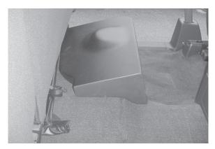
Flip up driver side rear seat and place enclosure on floor as shown above. Enclosure should be inside seat trim if the seat is in the down position.
