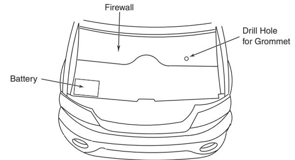
**Note:** To avoid any damage to parts inside engine compartment, drill from inside of vehicle using a short bit.
