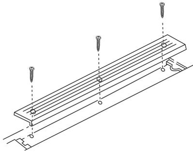
**19.** Using hardware provided, attach the mounting brackets to the enclosure as shown below. If installing in a 1999 or newer model, add rubber foot as shown below.
