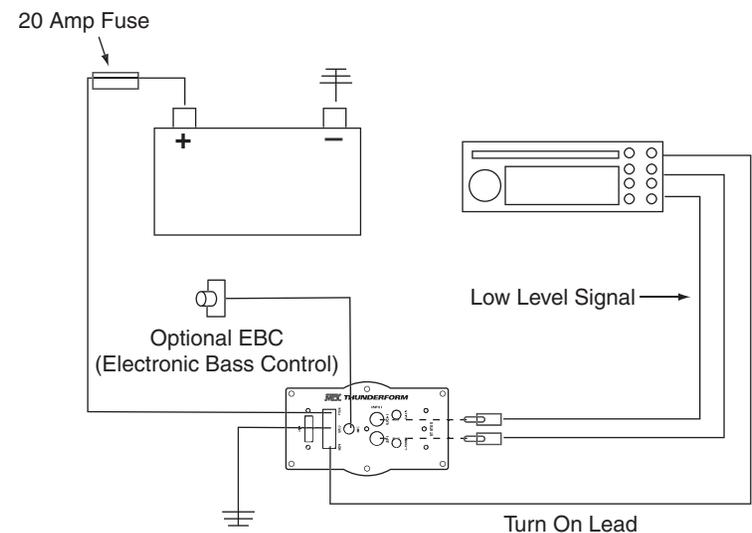
**Optional-** The EBC, or Electronic Bass Control, allows a remote bass control to be adjusted from the driver's seat.
