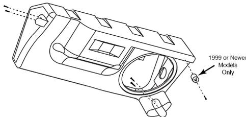
**20.** Using screws provided, install the enclosure into vehicle as shown below.
