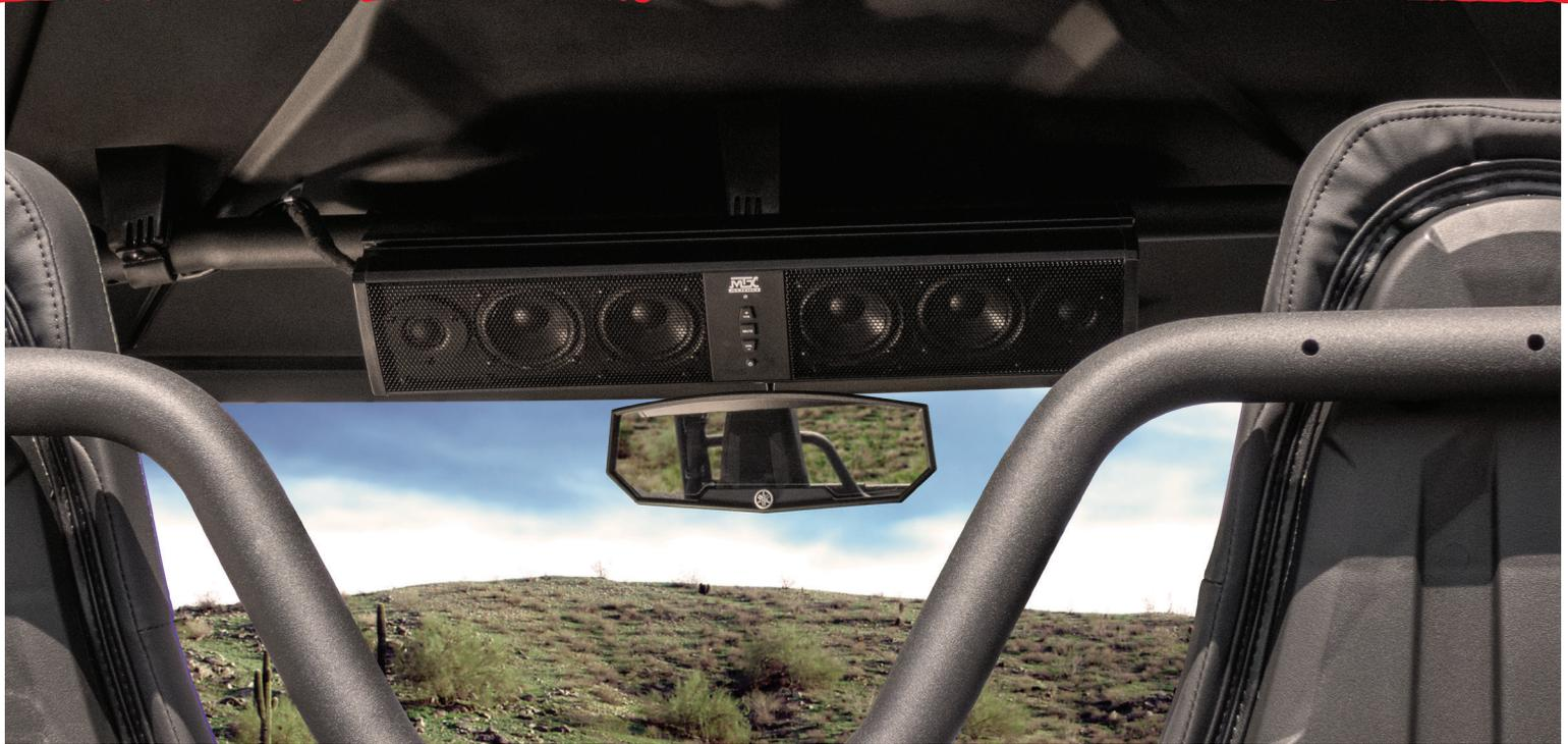
Our universal 6-speaker sound bars are a great choice when an overhead design isn't practical. With their multi-directional mounting system, they can be mounted almost anywhere on the vehicles roll cage. The internally amplified speaker system is available with an AUX input for music connection, or you can upgrade for added Bluetooth connectivity.
